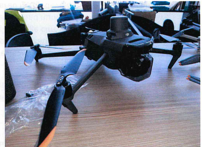
Drone with infra-red sensor and GPS guidance
